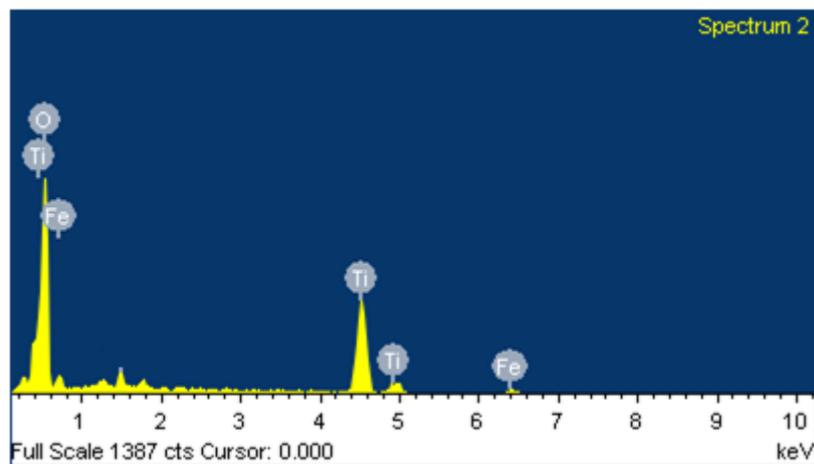
**Figure 4.** FESEM-EDAX data confirming Titania rich slag formation. [a].
