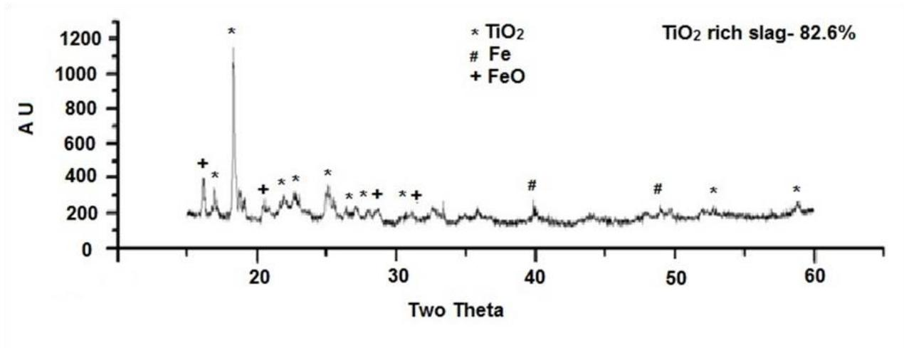
**Figure 3.** XRD results after microwave treatment of ilmenite.
