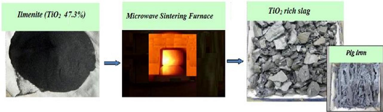
**Figure 1.** Schematic sketch for heating of ilmenite sample in a microwave furnace
