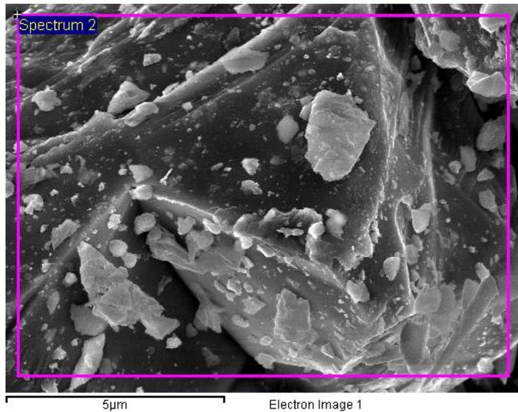
**Figure 4.** FESEM-EDAX data confirming Titania rich slag formation. [b].
