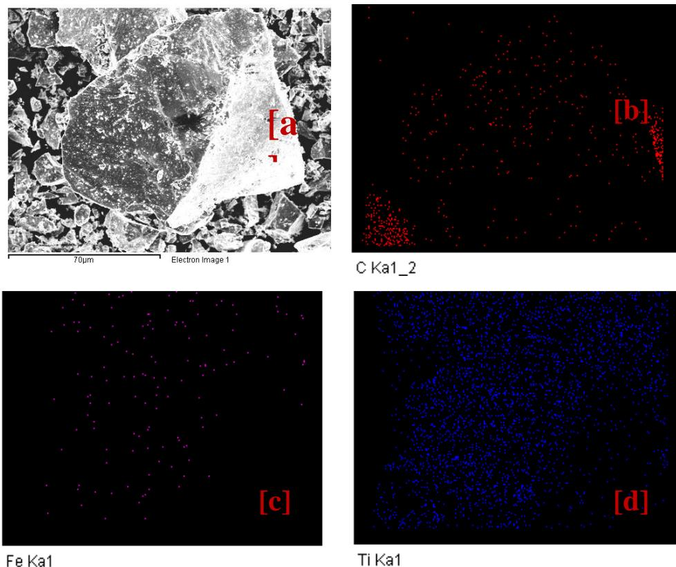
**Figure 5.** [a] FESEM of titania slag sample; image mappings of [b] carbon C [c] titanium Ti [d] iron (Fe).
