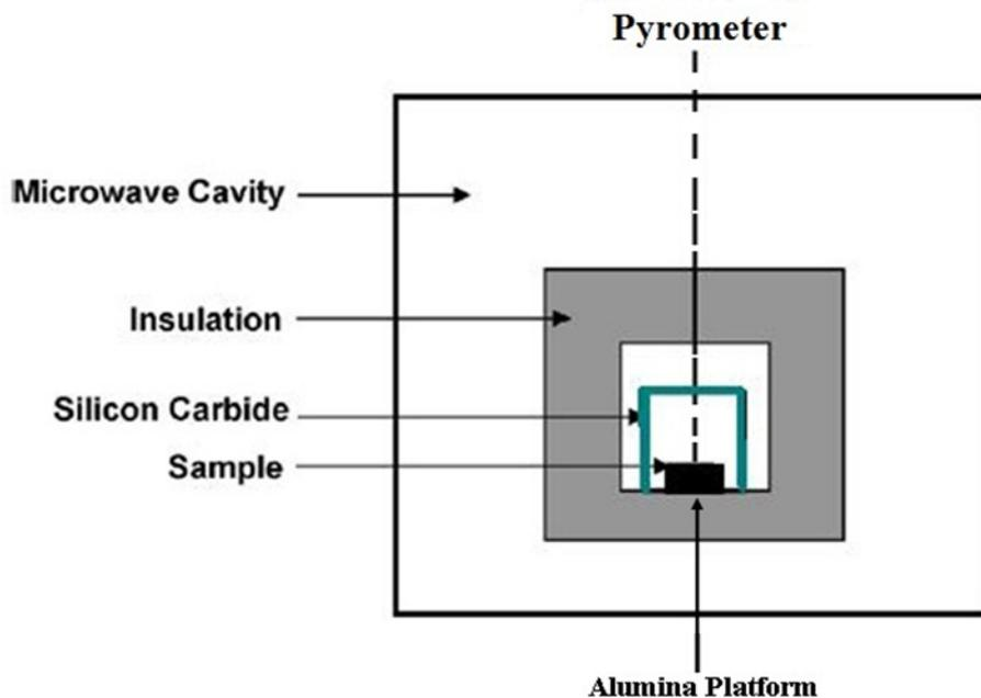
**Figure 2.** General schematic for microwave heat treatment process.
