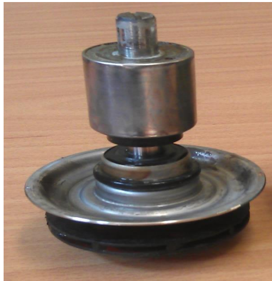
Figure 7. The inside of the pump, rotated by the water flow
