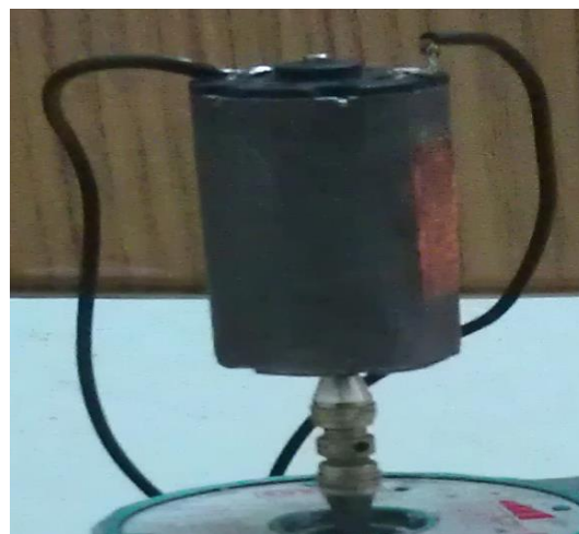
Figure 8. The picture of the DC motor used to generate electricity
