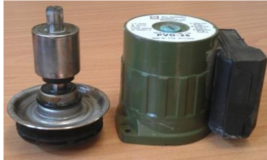
Figure 6. The circulation pump of a combi boiler
