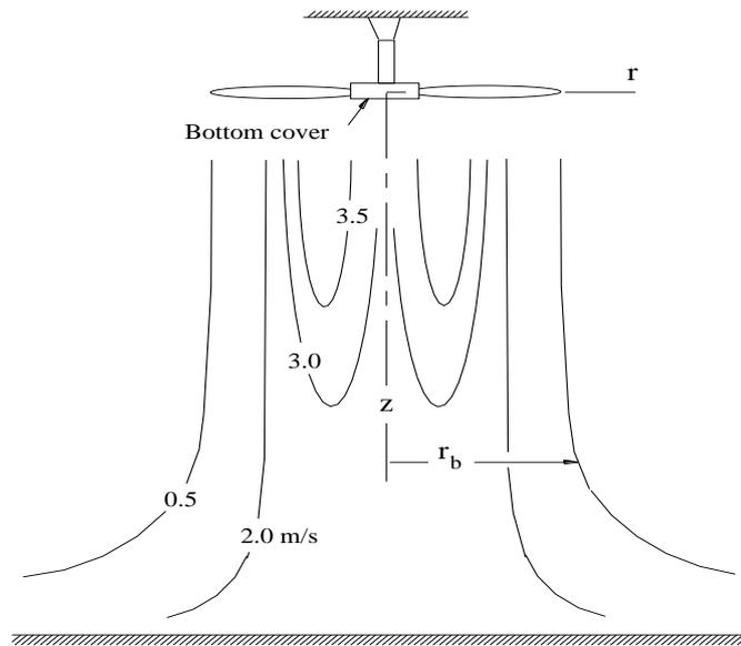
Fig. 1 Schematic of a ceiling fan and its isovels for axial velocity [7].
