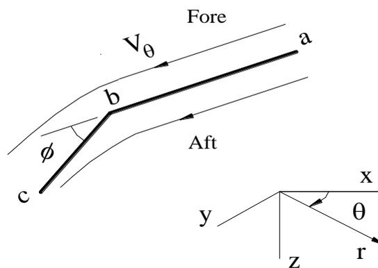
Fig. 2 Blade cross-section of a ceiling fan and geometrical axis.
