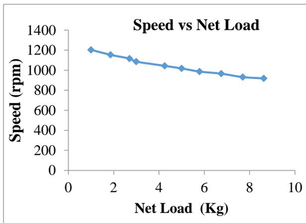
Fig 1. Effect of net load on speed, rpm
