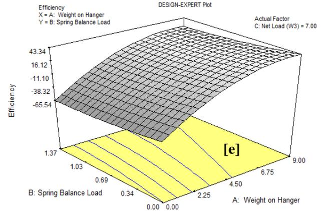
Fig 3 [Left Column] Optimized response surface plots for the experiments performed for Pelton turbine experiment showing (a) speed (rpm) (b) discharge Q (m<sup>3</sup>/ sec) (c) amount of input power (kW) (d) amount of output power (kW) (e) Efficiency (%)
